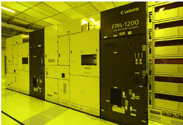
Nanoimprint semiconductor lithography equipment in use at Toshiba Memory
