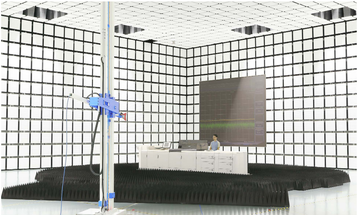
One of the largest semi-anechoic chambers in Japan where tests on large products can be carried out (→P116)
