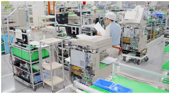
Remanufacturing in progress
