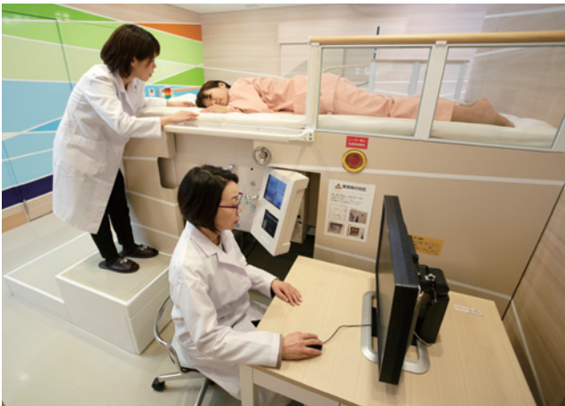
Photoacoustic Mammography captures images of blood vessels around tumorous tissue using laser radiation. If realized, it would enable nearly pain-free exams without exposure to X-rays.
