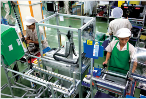
“Man-machine cells” production systems integrate processes where robots excel with processes that can only be performed by people to sharply enhance the productivity of cell production systems, enabling further improvement in quality and productivity. (Canon Hi-tech (Thailand) Ltd.)
