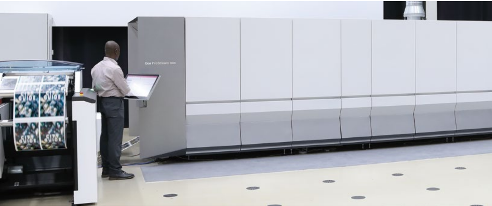
The Océ ProStream 1000 continuous-feed color printer for the graphic arts market can print on offset coated paper thanks to Océ's newly developed ink set and ColorGrip technology. (Océ, Germany)
