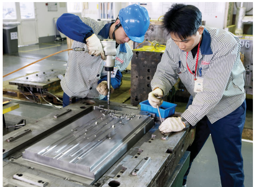
In-house production of a mold at Canon (Suzhou) Inc.
