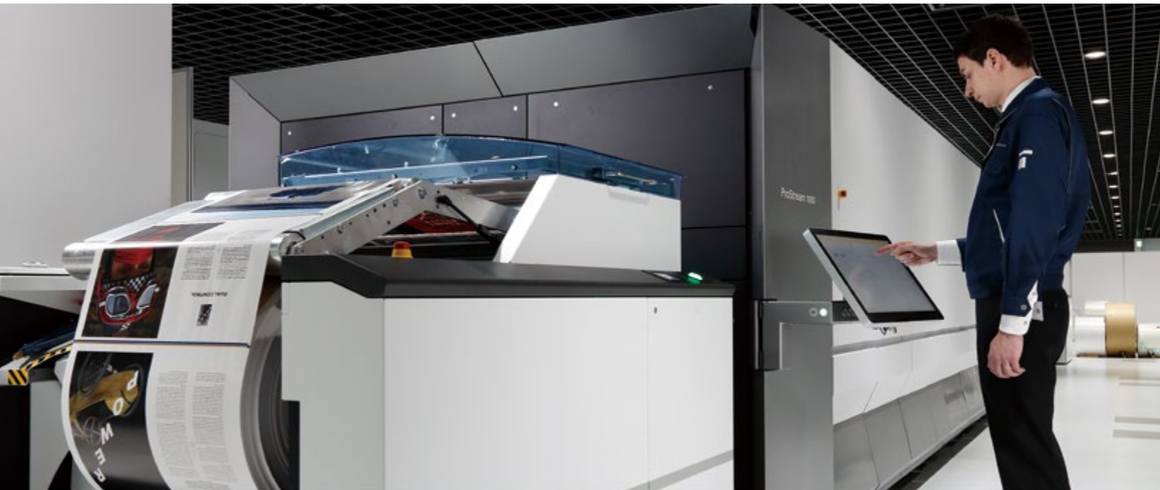
The continuous feed press ProStream 1000 can print on offset coated paper thanks to Canon's newly developed ink and ColorGrip technology.
