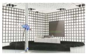
EMI measurement of products in a semi-anechoic chamber
