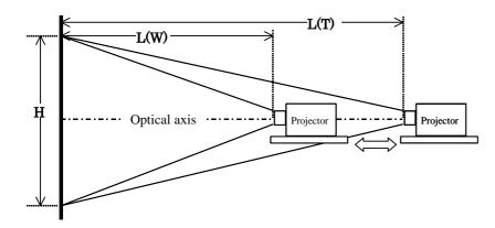
Image of height H is projected in the range from the shortest distance L (W) to the longest distance L (T).
