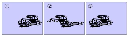
In this example, a composite image ② appeared when an object moved from right to left, which is a combination of the frames before and after the movement.
