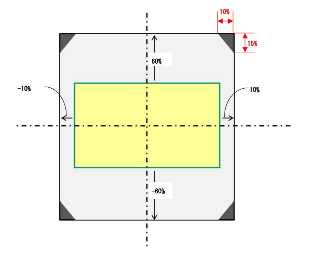
\* Moving the image outside the guaranteed optical performance range may cause shade to appear in the corner area of the image. (e.g., 60% vertical, 10% horizontal → the upper right corner of the image becomes dark)
