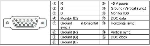
For pin 9, 12, and 15, use a cable that supports conduction line.
