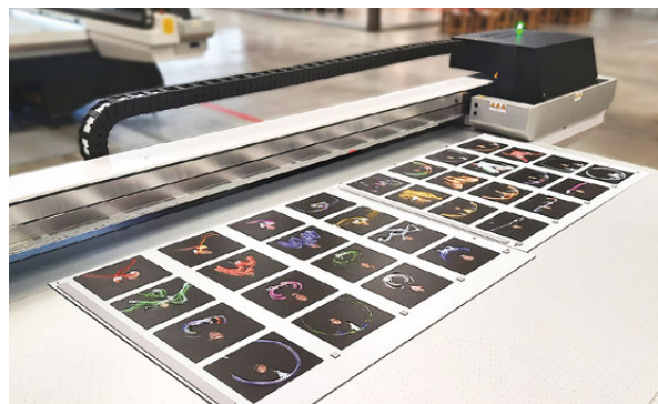
Production of the "FUGA" photographs using elevated printing technology
