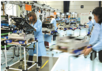
*Cell production The cell production system makes conventional conveyor-belt based production lines obsolete. Small teams of employees assemble products together, with each team member taking responsibility for a greater number of the production processes.
