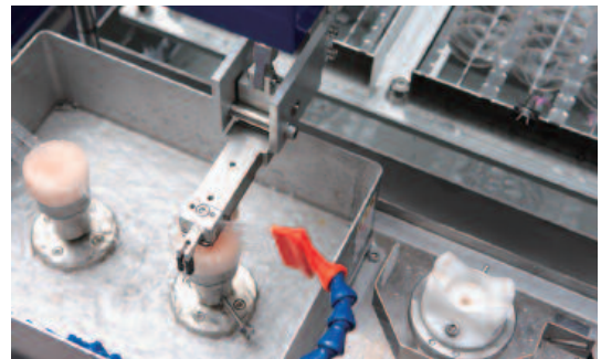
Lenses are cleaned at Oita Canon with purified and reused wastewater from the plant
