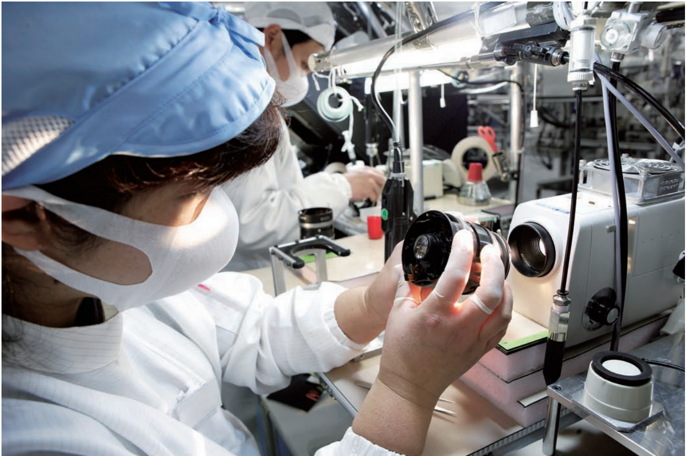
Cell production of interchangeable lenses for SLR cameras at Oita Canon, Japan
