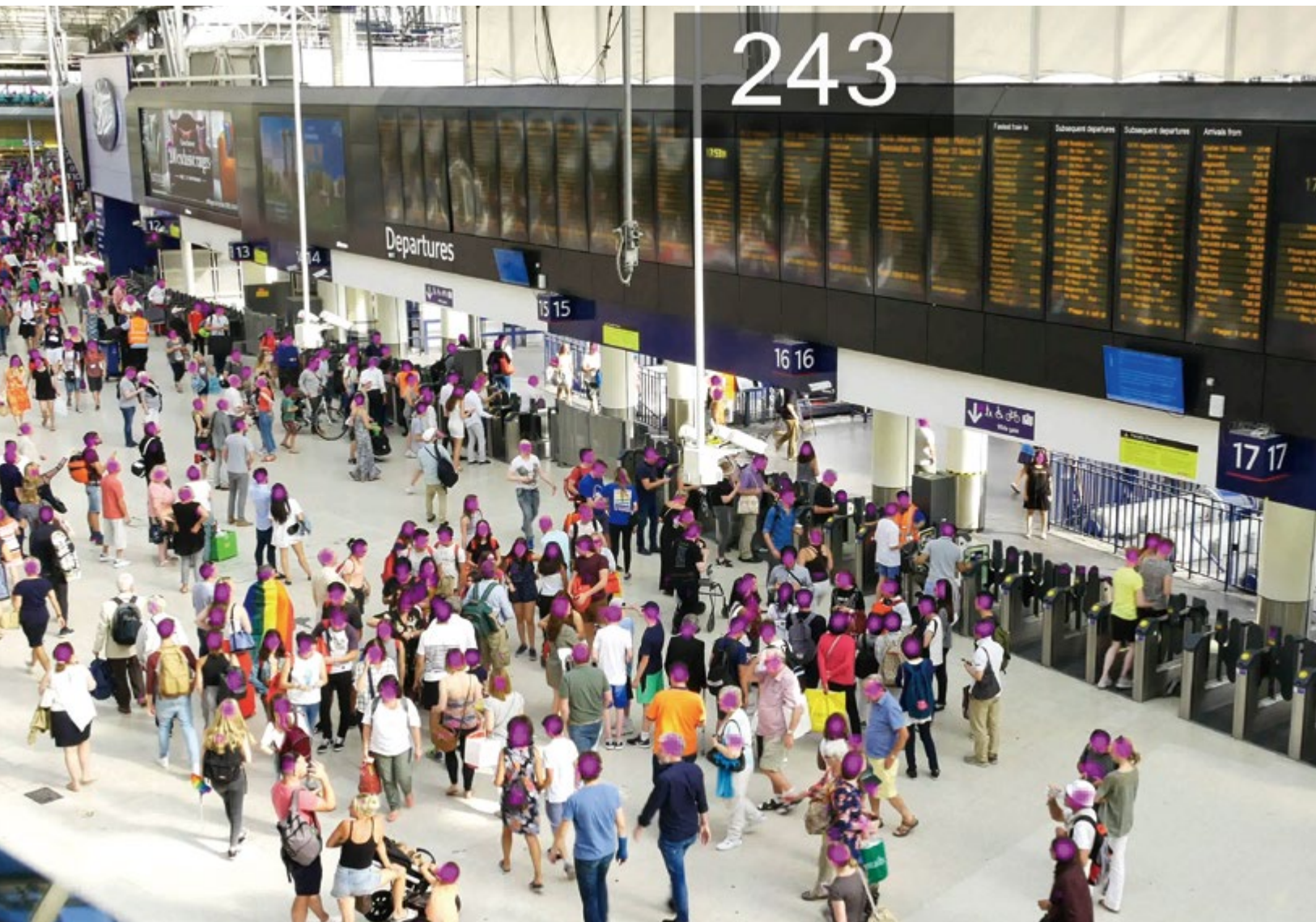
Canon's crowd people counting technology utilize AI to detect and count the number of heads, making it possible to count the number of people in a crowd in real time.
