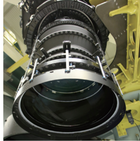
Wide field corrector installed in the HSC
