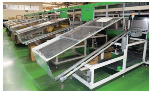
Automated toner cartridge sorting system
