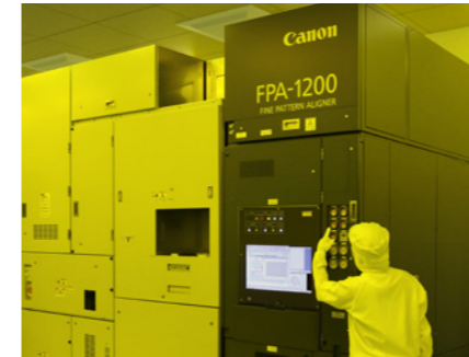
Canon's semiconductor manufacturing equipment using nanoimprint lithography technology revolutionizes the circuit pattern transfer process.
