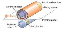
The use of a ceramic heater that heats up quickly and a fixing sleeve that transfers heat efficiently allows for localized heating of the fixing point and instantaneous heat transfer. No excess electricity is consumed in standby mode, enabling a shorter warm-up period.
