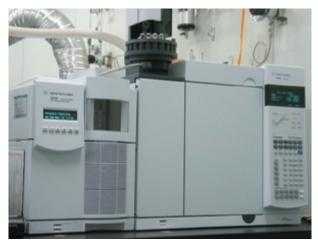
Gas chromatograph mass spectrometer used to measure chemical substances emitted from products
