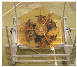
Hexagonal-shaped segment mirrors making up the primary mirror
