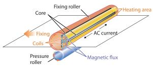
An electromagnetic induction heater induces an eddy current when magnetic flux passes through metal coils, causing the fixing roller to emit heat. In this way, overall heat efficiency is improved and energy consumption is reduced.
