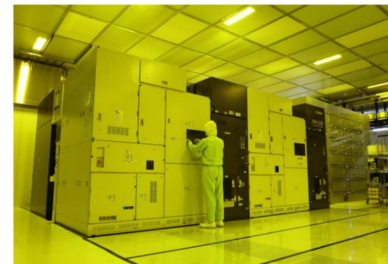
Semiconductor lithography equipment using nanoimprint technology installed at Toshiba Memory
