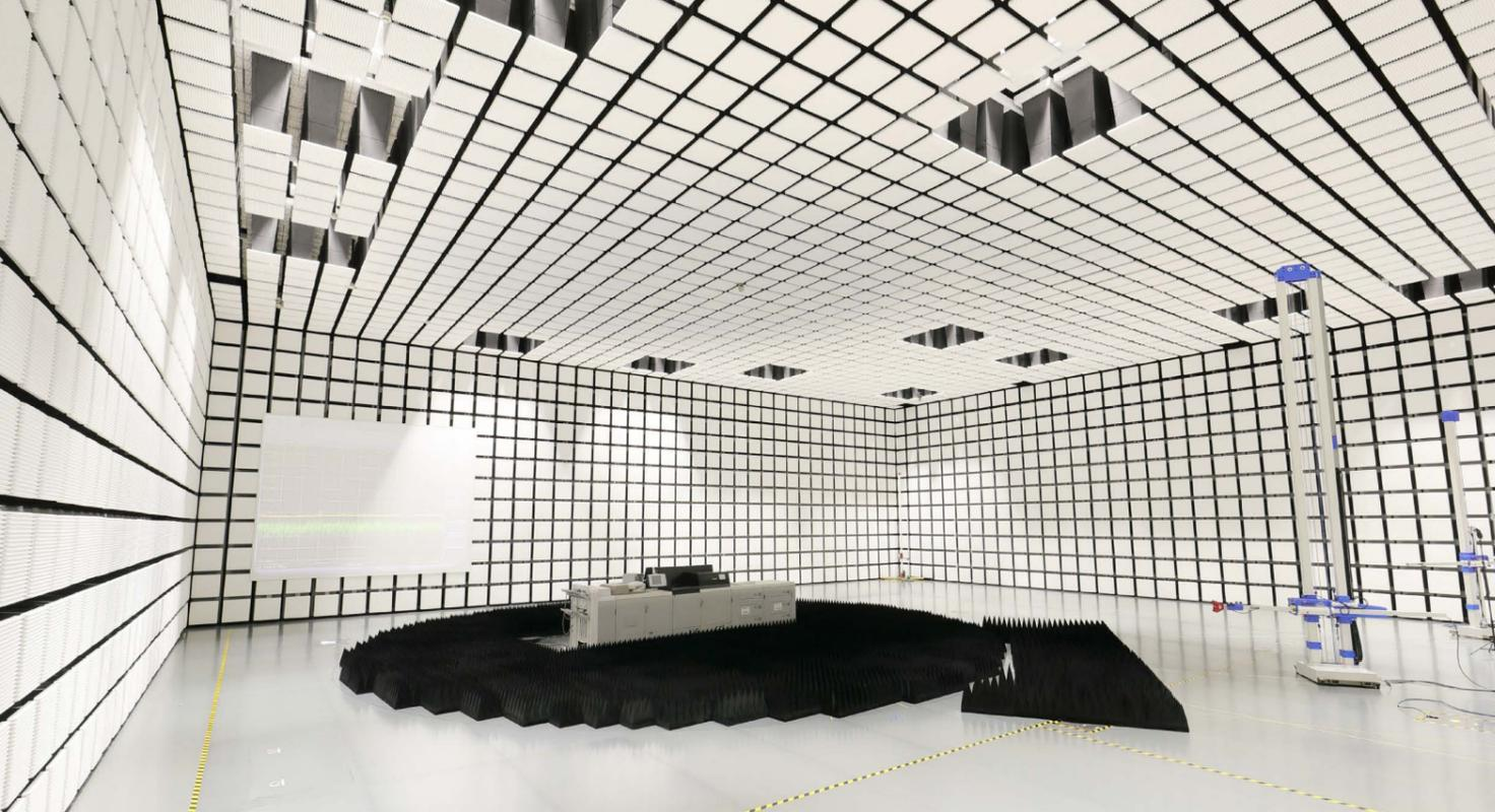
One of the largest semi-anechoic chambers in Japan where we carry out tests on large products (→P112)
