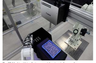
The 3D Machine Vision System can pick out parts from a pile
