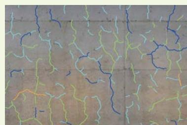
AI-based detection of structural cracks
