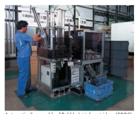
Automatic disassembly of Bubble Jet ink cartridges (CROC)
