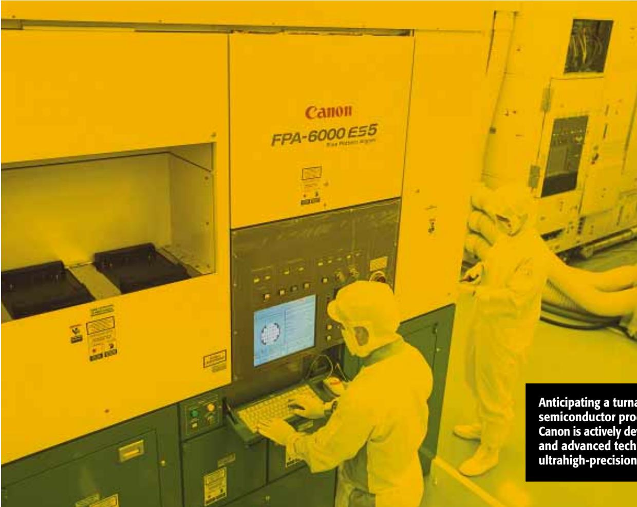
Anticipating a turnaround in demand for semiconductor production equipment, Canon is actively developing new steppers and advanced technologies to expose ultrahigh-precision circuit patterns.
