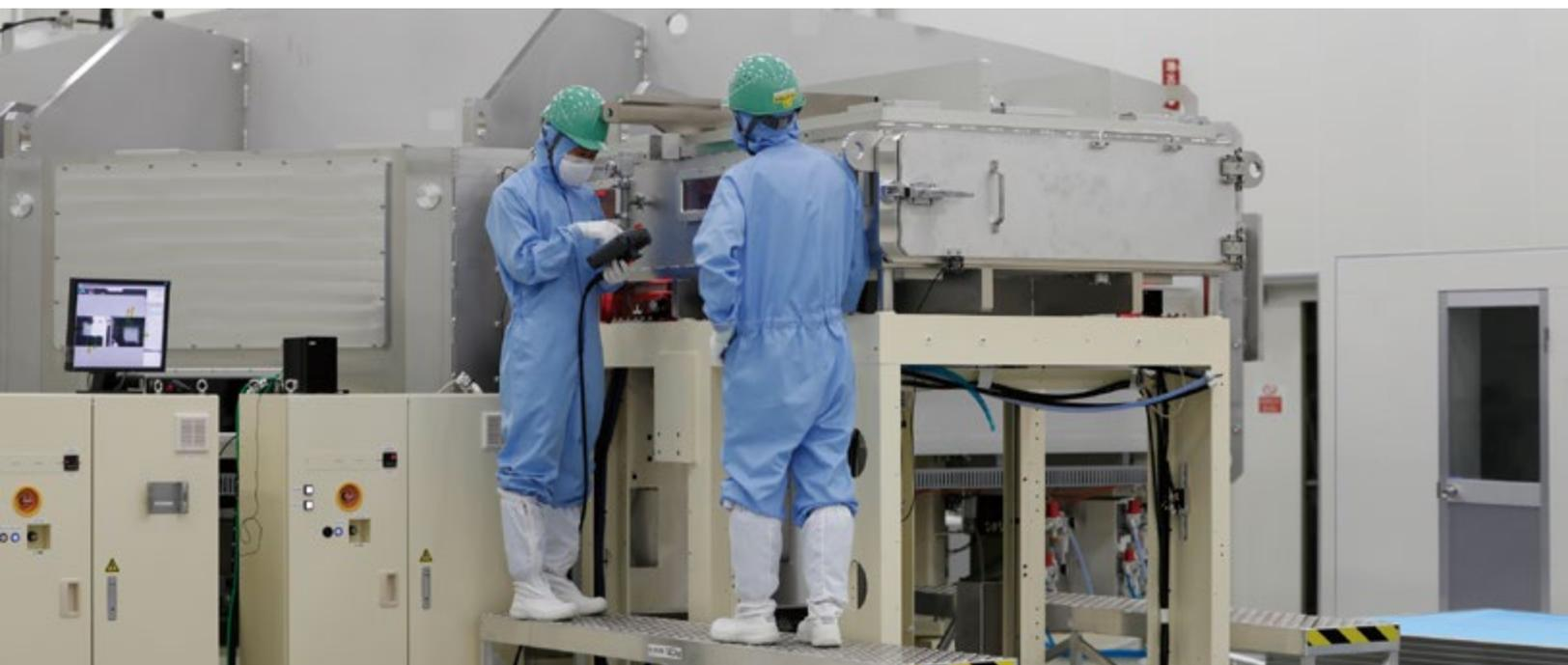
Canon Tokki produces OLED panel manufacturing equipment with high-level technologies, including vacuum evaporation technology for depositing organic materials onto panel substrates in a vacuum and automated supply lines for glass substrates.
