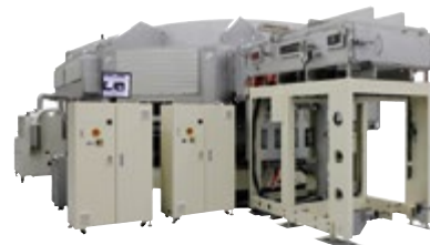
Organic LED (OLED) panel manufacturing equipment
