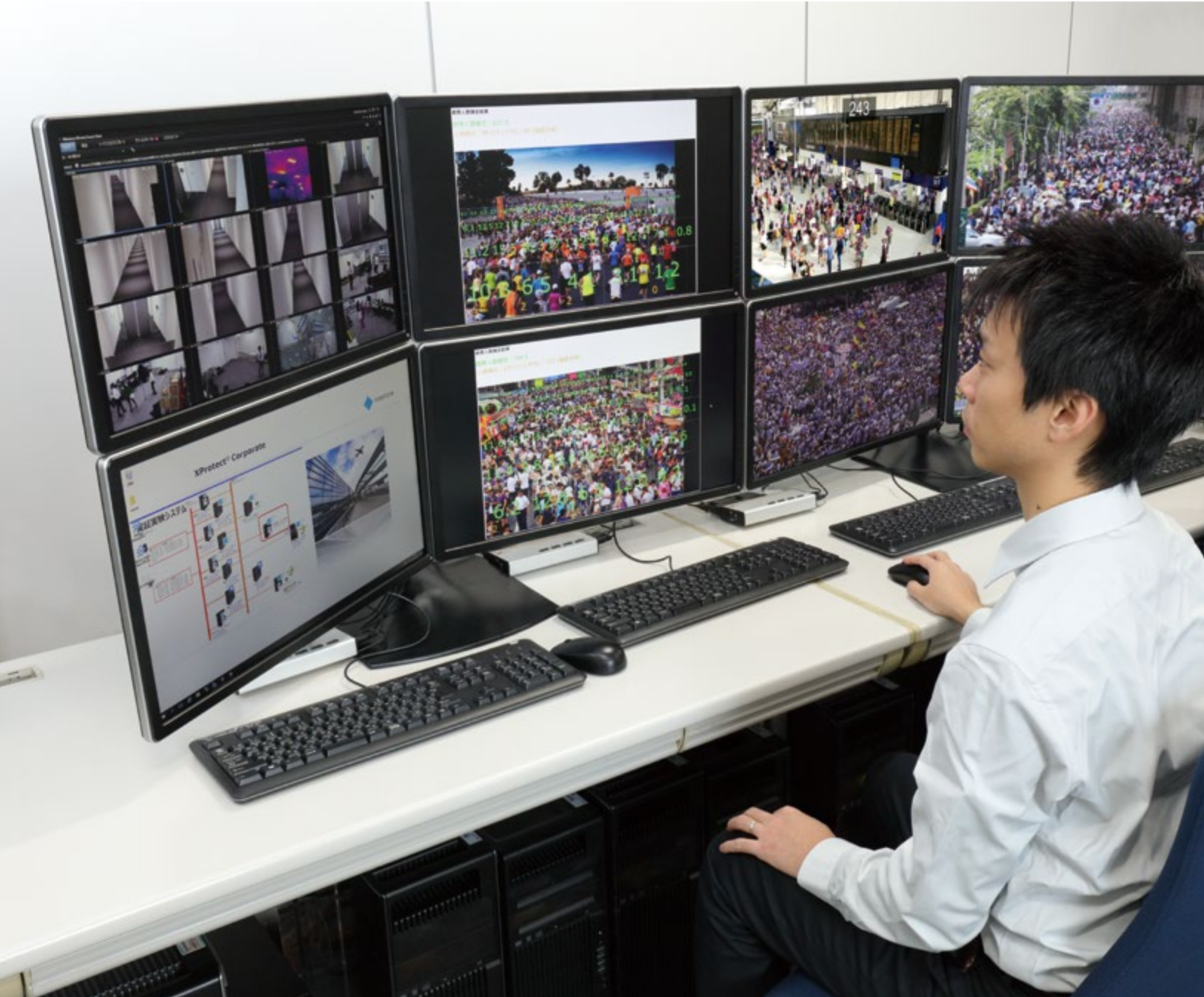
Canon's crowd people counting technology utilizes AI to detect and count the number of heads, making it possible to count the number of people in a crowd in real time.
