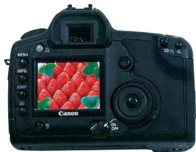
Canon plans to equip digital cameras and camcorders with OLED displays (prototype)
