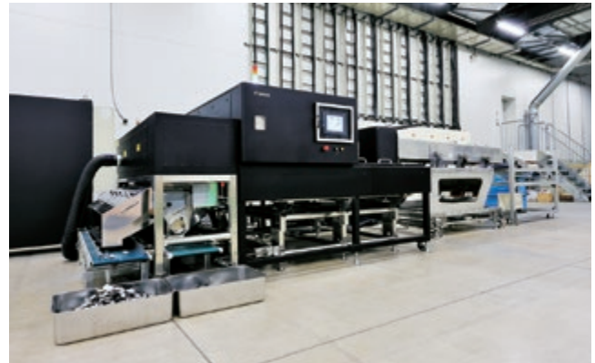
High-precision sorting equipment capable of measuring black plastic pieces, which are difficult to identify
