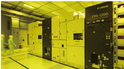
Nanoimprint lithography equipment being used for mass production verification at KIOXIA Corporation
