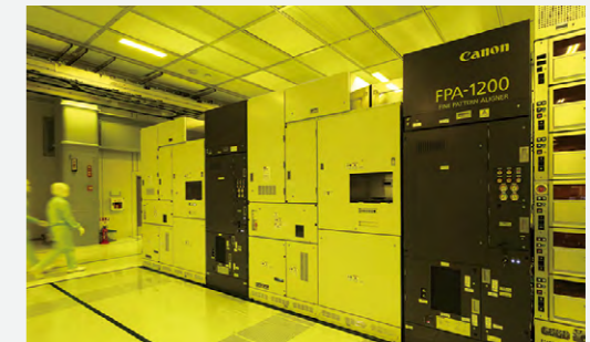
Nanoimprint lithography equipment being used for mass production verification at KIOXIA Corporation
