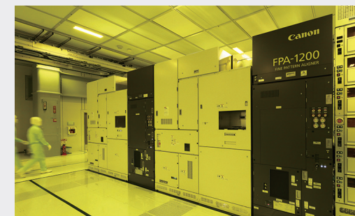
Nanoimprint lithography equipment being used for mass production verification at KIOXIA Corporation
