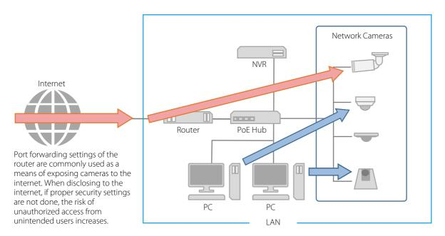
Networks that allow external access are highly convenient, but at the same time the risk of unauthorized access to devices on the network increases. Therefore, in such a network configuration as illustrated above, it is important not only to implement the countermeasures described in this document, but also to secure measures to the entire system such as authentication of each device and encryption of each communication on the network.
