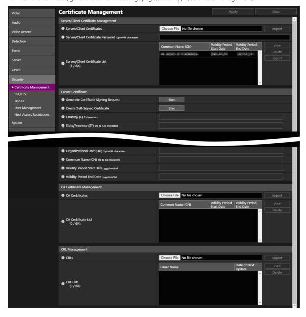
Encrypting communication by HTTPS connection is set in [Security] > [SSL/TLS] on the camera's setting page.
