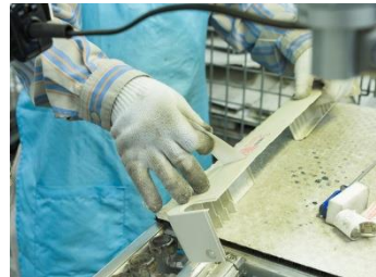
Check plastic type, remove foreign matter/labels
