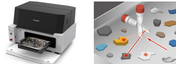
(Left) Raman Plastic Analyzer TR-A100 (Right) Canon's high-precision galvanometer scanner sequentially irradiates multiple plastic pieces arranged on a tray with a laser, and the material is identified by spectroscopically analyzing the material-specific Raman scattered light generated in the process.
