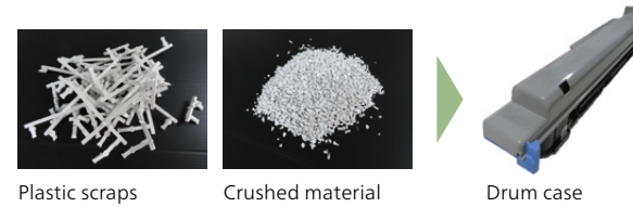
Plastic scraps Crushed material Drum case 100% recycled-material drum case made from plastic scrap * Excluding color masterbatches
