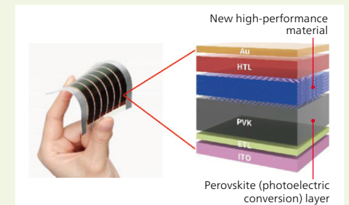
(L) Perovskite solar cell (R) Structure of perovskite solar cell with newly developed high-performance material
