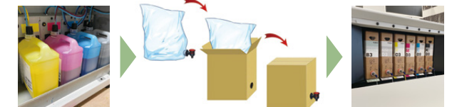
Mechanism of the Bag-in-box System
