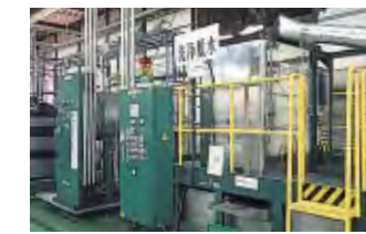
Line for cleaning and removing foreign objects from plastic
