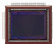
CMOS sensor with approximately 250 megapixels
