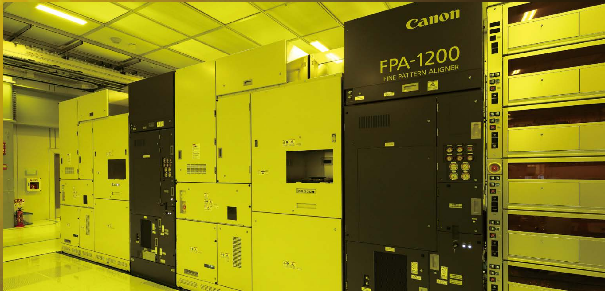
KIOXIA Corporation / Canon's nanoimprint semiconductor-manufacturing system is currently being studied mass production at KIOXIA's Yokkaichi plant
