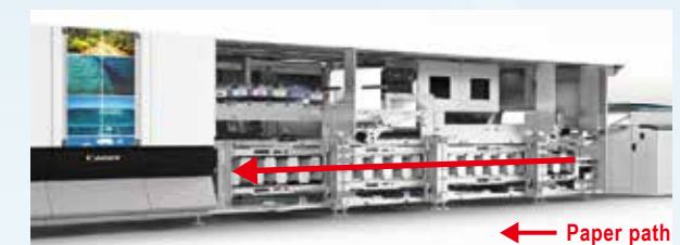
Inside the ProStream 1000 (Non-contact ink drying technology)
