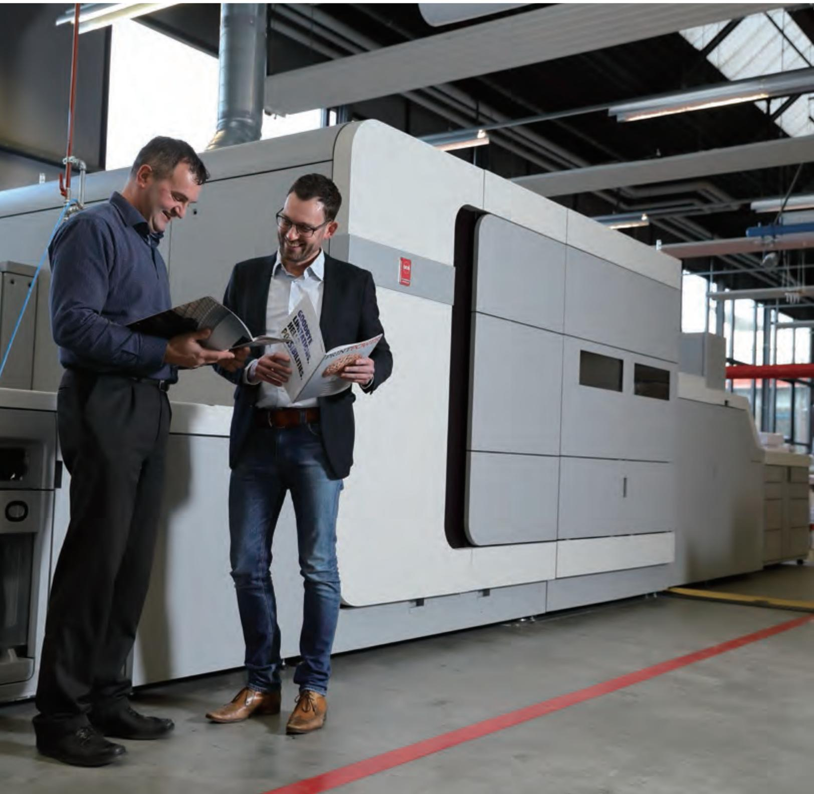
The Océ VarioPrint i300 sheet-fed inkjet color press, which is a high-speed commercial printer, uses Océ's unique paper transport technology to achieve stable, high-speed output. Océ's proven technologies enable printing on a range of media, including coated paper, to meet diverse needs in commercial printing. (Customer Experience Center Venlo, Netherlands)
