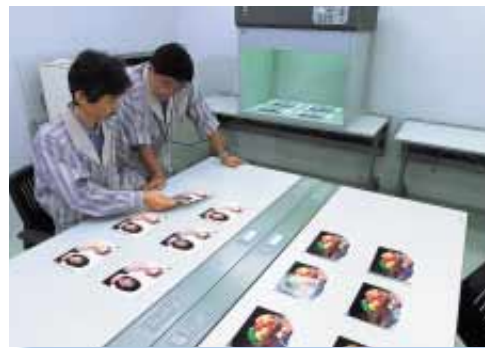
Image matrix assessment is used to define colors for the color management database.
