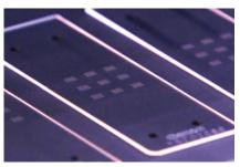
Canon established DNA chip production method using its Bubble Jet printing technology
