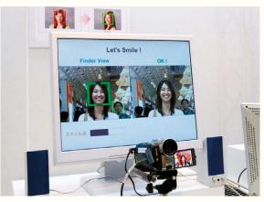
Intelligent Vision system Our automated Intelligent Vision system can distinguish faces and recognize facial expressions, including smiles. The system's embedded intelligence can be programmed to detect faces and automatically snap a photo the instant a smile appears, and pause when blinking eyes are detected.
