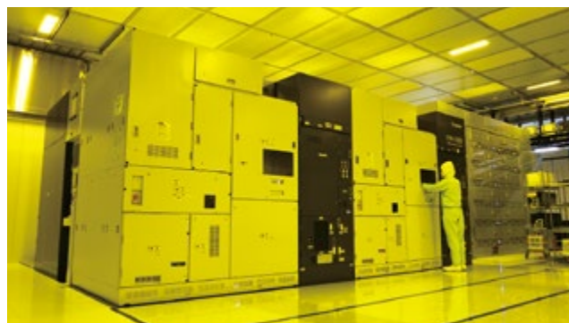
Mass production verification of nanoimprint manufacturing equipment is underway at Kioxia's Yokkaichi plant. (Japan)
