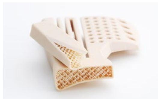
Complex ceramic lattice structure in hollow shapes
