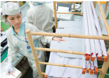
The cell production system helped to improve employee motivation and to reduce CO 2 emissions through the elimination of conveyor belts (Photo: an example of intelli-tech at Canon Vietnam)
