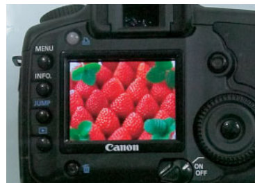
Organic LED displays achieve high luminance while also offering high definition, excellent color reproduction, and high image quality from any viewing angle (prototype)
