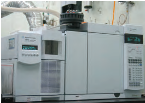
Gas chromatograph mass spectrometer used to measure chemical substances emitted from products
