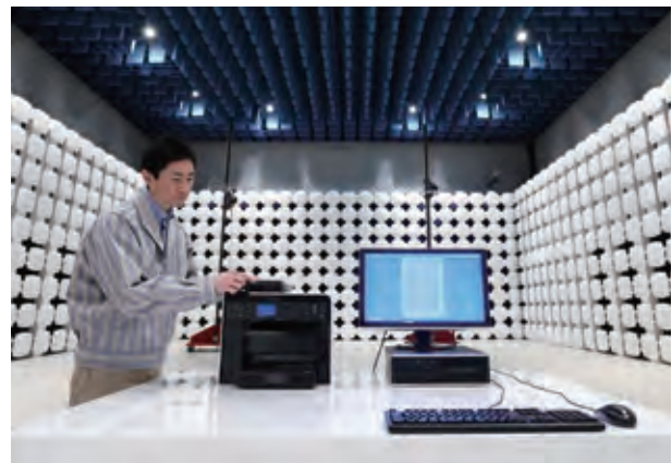
EMI measurement of products in an anechoic chamber
