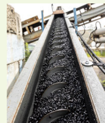
Recycled toner pellets used as asphalt additive
